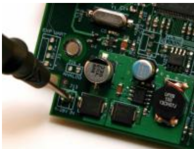
Ground Probe Point
